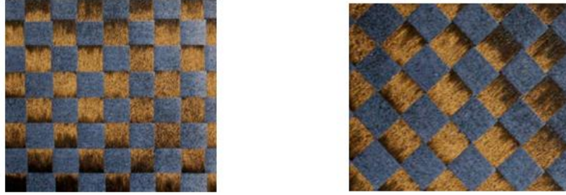
Figure 18. Orientation of the woven fiber in the outer layer, optimized for bending at 0° and 90° (left) and for torsion at 45° and -45° (right).
